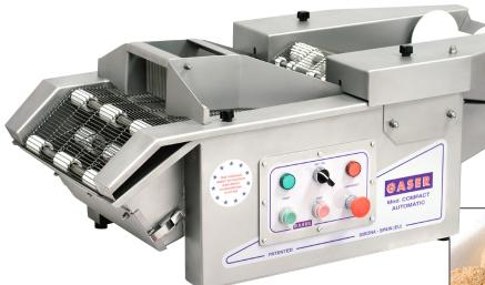
Compact model, a tabletop machine for small productions; specifically indicated for meatball and croquette manufacturing, as well as other similar products of small size.
